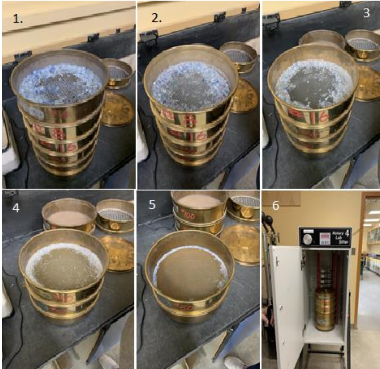
Figure 1: Spike sample results post mechanical sifting. Evident is the separation of plastics decreasing in size at each sieve, clockwise 1-5; Rotary Lab Sifter in 6 (Photos: Q. Dartnell).
