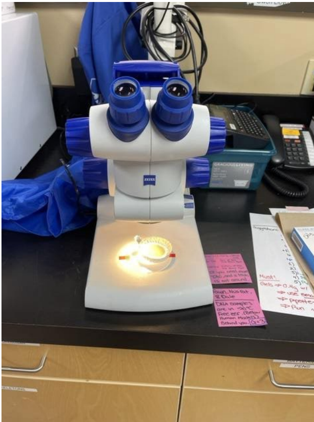
FIGURE 9: DISSECTING MICROSCOPE USED TO COUNT MICROPLASTICS AT 40 X MAGNIFICATION.
