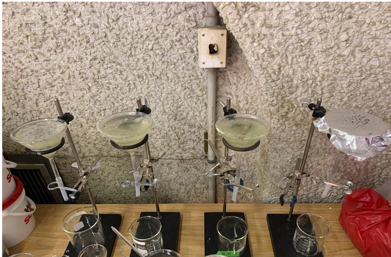
Figure 7: Funnels sitting in ring clamps with clamped hoses attached to stem. Solutions have been poured into funnels for density separation to occur (Photo: Q. Dartnell).
