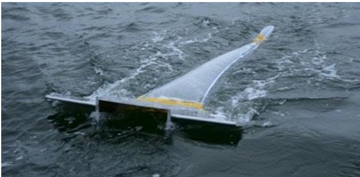
Figure 2: Manta Trawl being towed in water; water can be seen entering the central opening and passing through the netting with a collection point at the end (Photo: Microplastics Okanagan).
